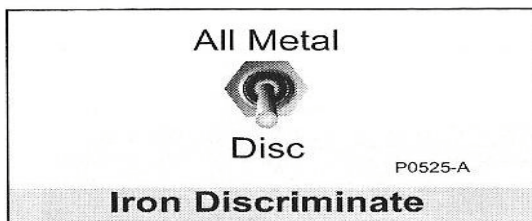
Figure 4.18 All Metal/Disc switch
